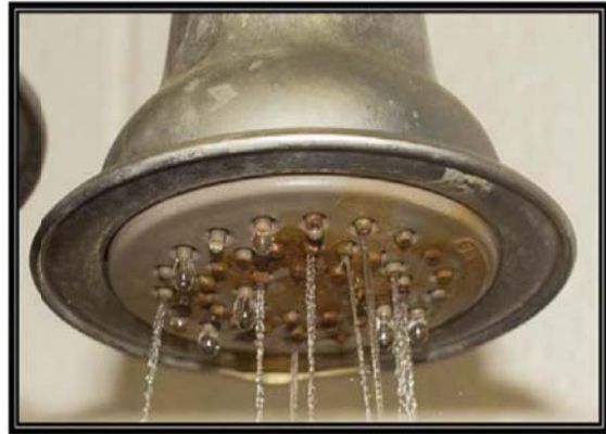
Showerhead with hard well water showing spray pattern. Battelle testing for Water Quality Association.
