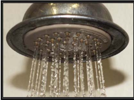
Showerhead with soft well water (<1 grain per gallon) showing spray pattern. Battelle testing for Water Quality Association.
